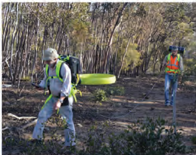
■ Greg Street (left) and Andrew Duncan walk their portable Loupe TEM system through terrain inaccessible to other modes of transport.
