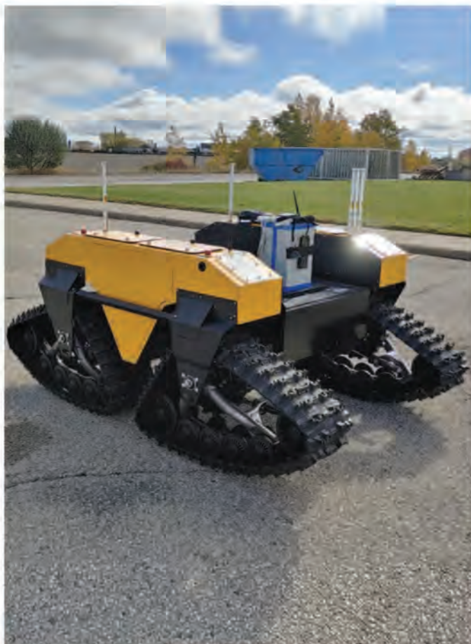
■ The Scintrex RG-1 remote operating gravity meter is deployed on various Clearpath autonomous and remotely operated all-terrain vehicles. CREDIT: SCINTREX LIMITED
