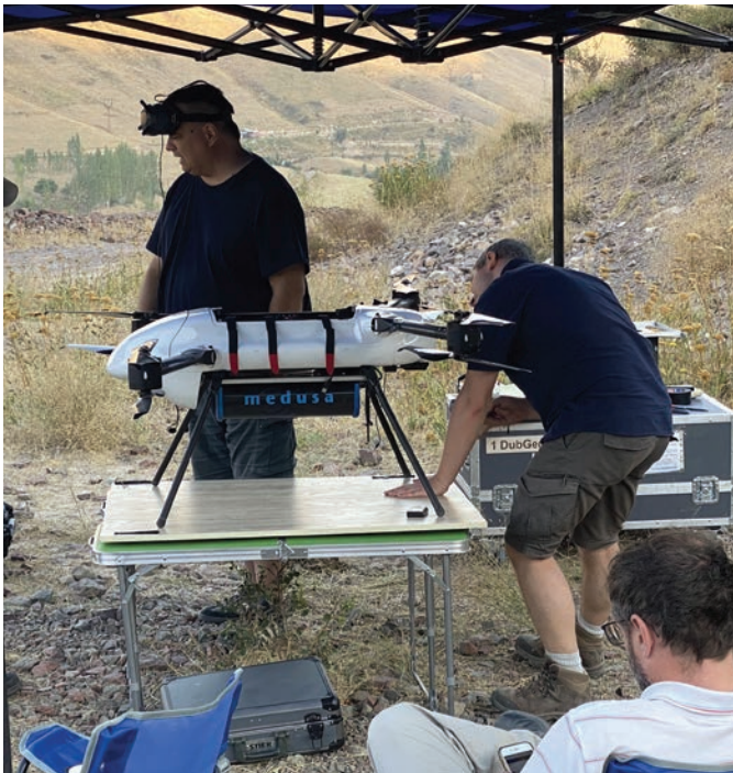
■ BGR field team mounting a MS-700 under their drone in Uzbekistan CREDIT: MEDUSA RADIOMETRICS BV
