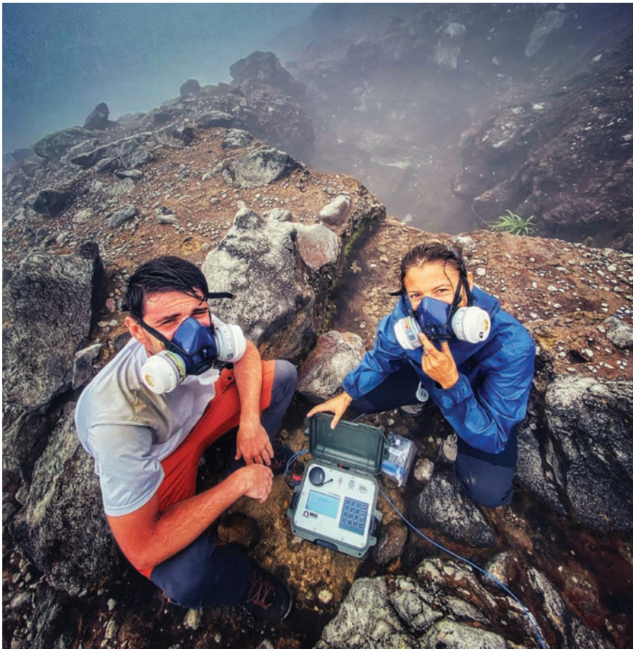
■ A FullWaver unit installed on top of La Soufriere active Volcano, Guadeloupe, West Indies. CREDIT: IRIS
