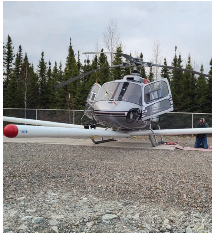
■ Tri-Boom Gradiometer Installed on Astar CREDIT: TERRAQUEST
